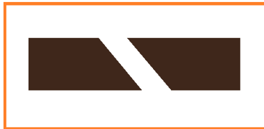
Fig. 10. Connecting the finishing strips front-to-front.
