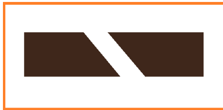
Fig. 11. Connecting the finishing strips front-to-front.
