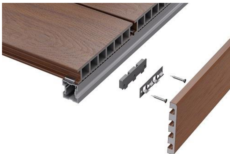
Fig. 10. Mounting the finishing strip.
